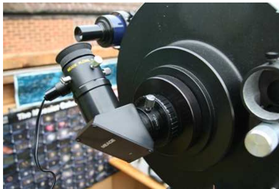
Fig. 1 – Diagonal & eyepiece set up used for Polar Alignment
