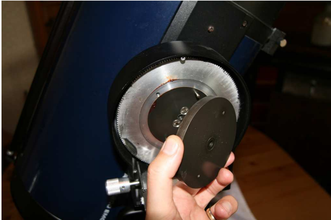
Figure 22 – Lift off the locking plate
