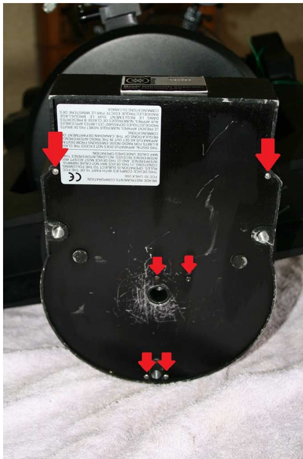
Figure 3 – Remove the six rear panel screws (arrowed)
