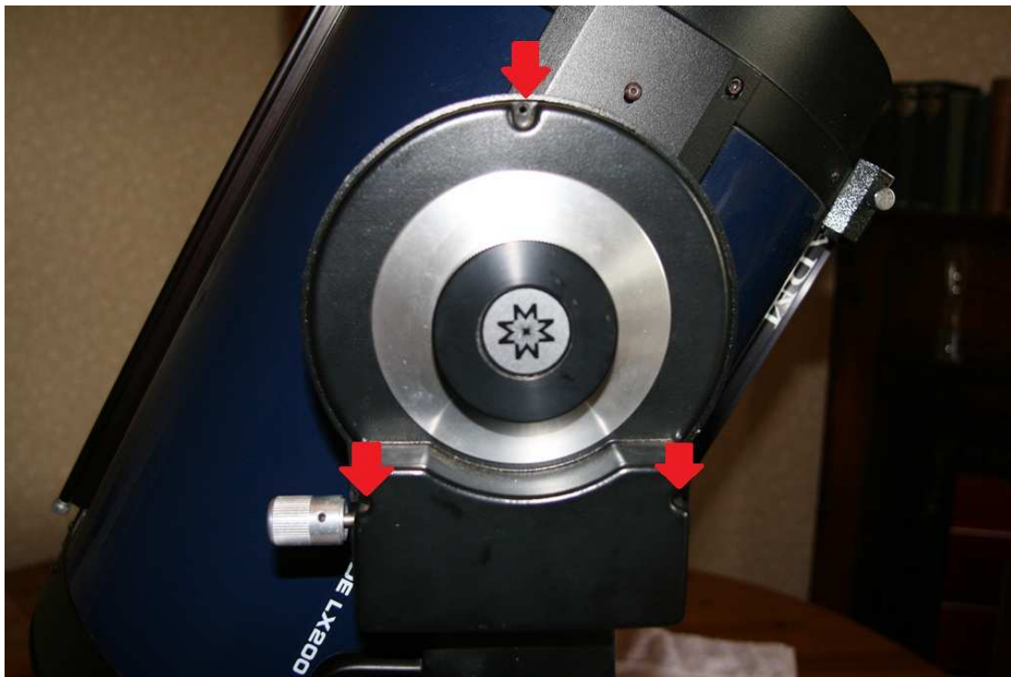
Figure 19 - Remove the three Dec housing screws (arrowed)
