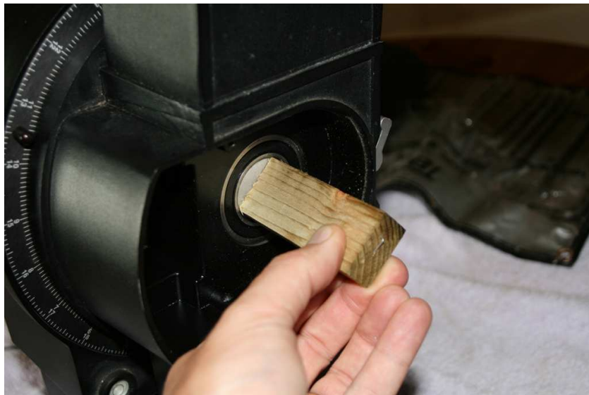
Figure 9 – Position a piece of wood or similar (ensure no contact on the bearing)
