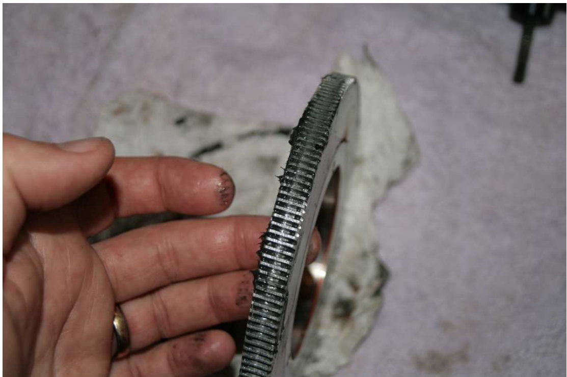
Figure 25 – The Dec gear wheel close up (before cleaning)
