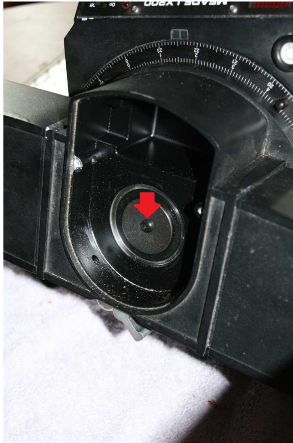
Figure 8 – Remove single screw (arrowed)
