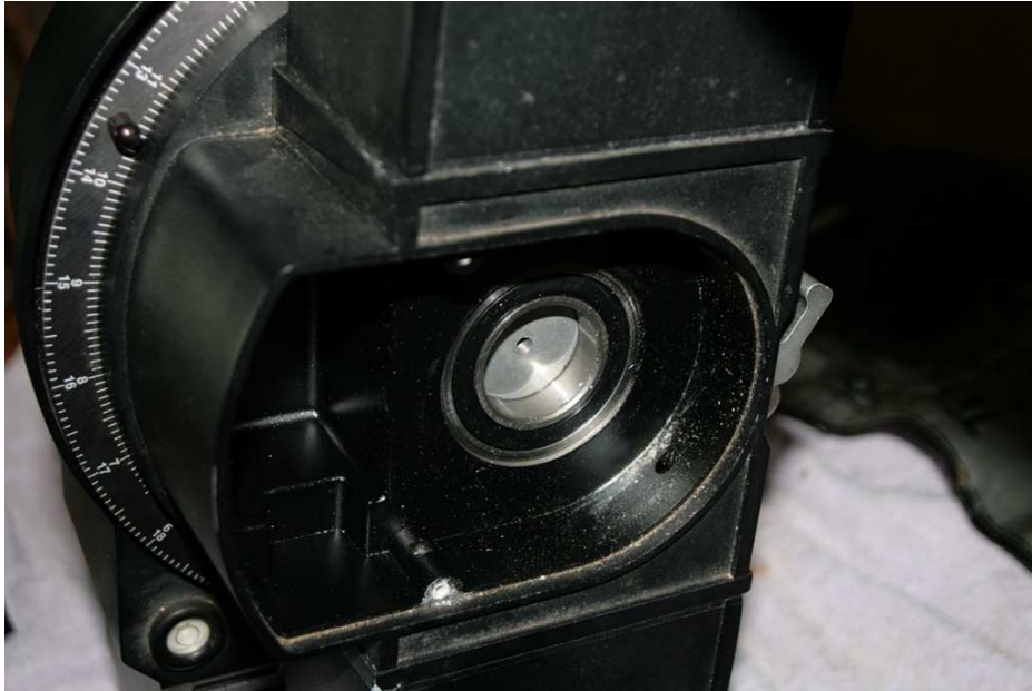
Figure 10 – RA shaft is moving out
