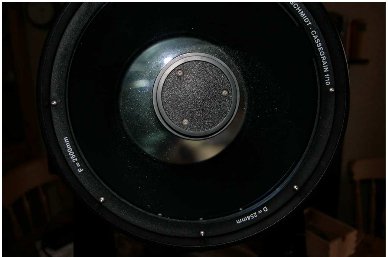
Figure 26 – Before cleaning – loads of dirt on the plate
