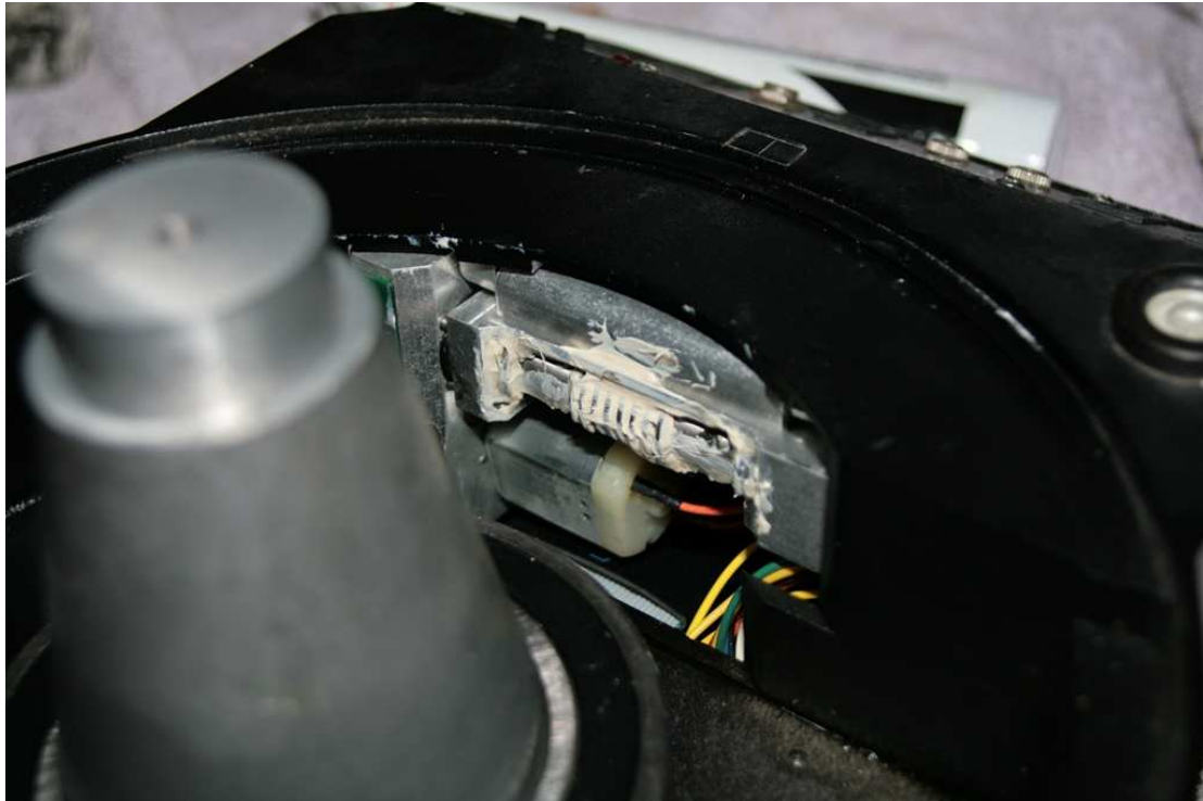
Figure 18 – RA work wheel cleaned up and re-greased
