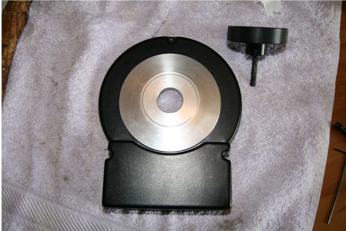
Figure 20 – The Dec locking wheel and cover removed
