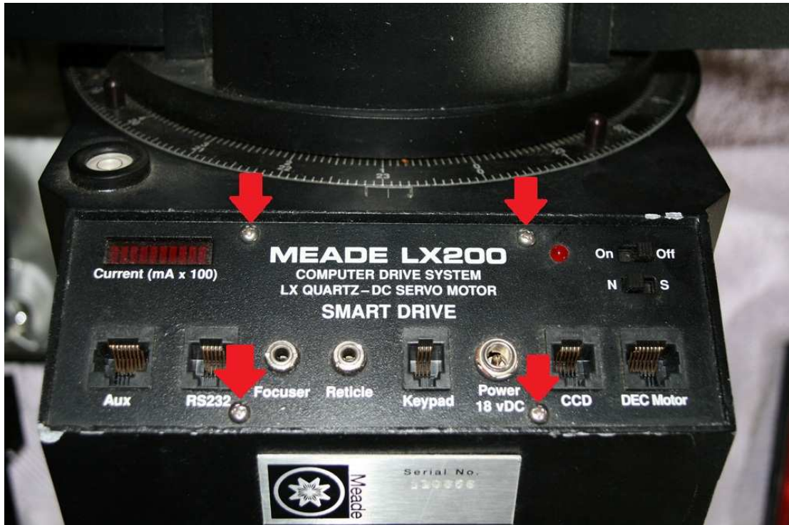
Figure 4 – Remove the four front panel screws (arrowed)
