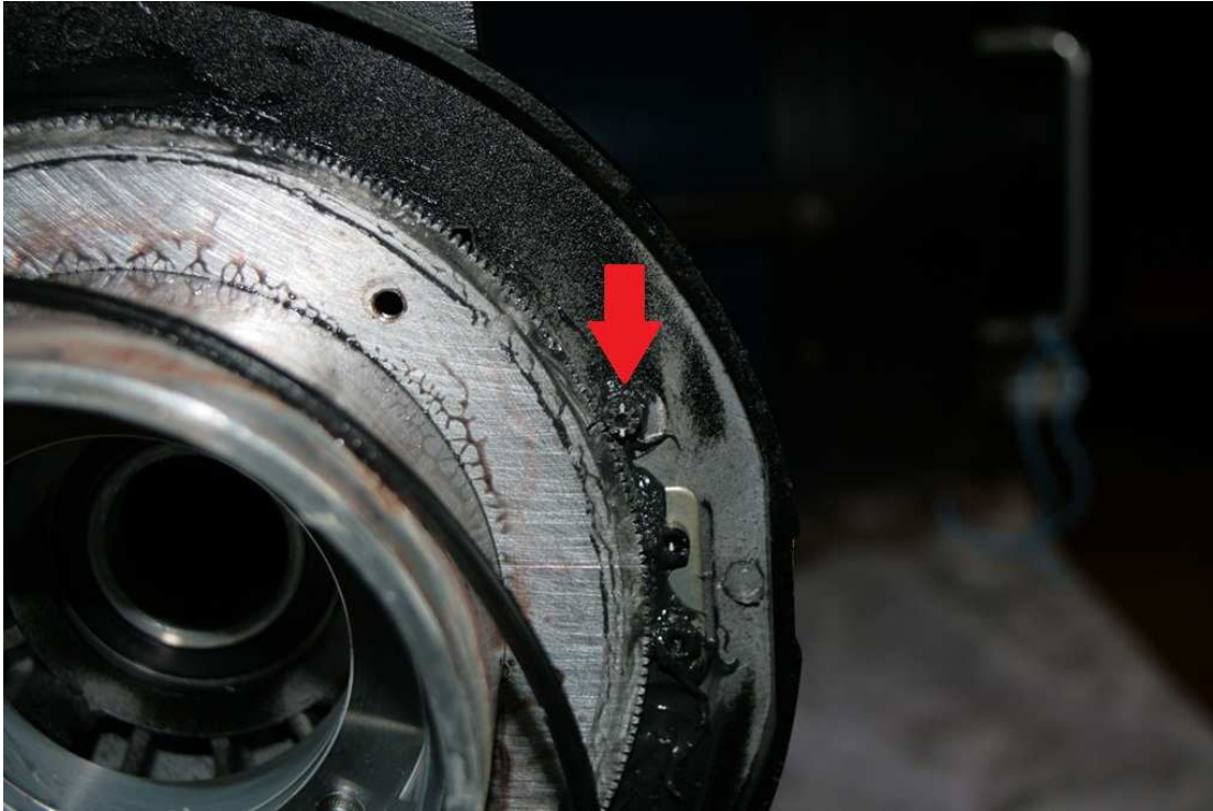
Figure 14 - RA slow motion control gear assembly (before cleaning)
