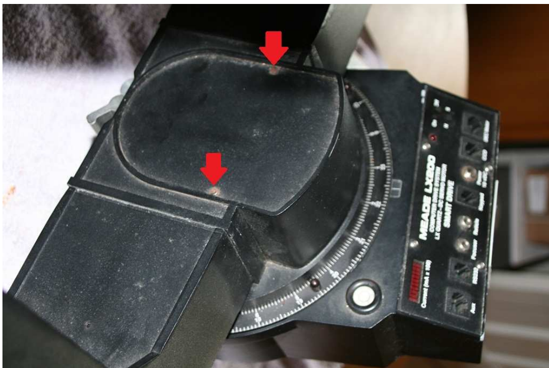
Figure 7 – Remove cover plate two screws (arrowed)
